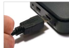
**Step 1C** Otherwise, get an HDMI cable from the MyWirelessTV 2 Kit. Plug one end into the **HDMI Input** port on the back of the transmitter.
