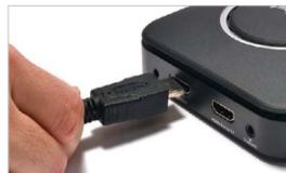
**Step 1D** Plug the other end of the HDMI cable into the HDMI port on the source device.
