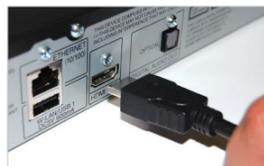
**Step 2A** Get the power supply from the MyWirelessTV 2 Kit. Plug the smaller end of the power supply into the 5VDC port on the back of the transmitter.
