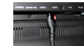
**Step 3C** Plug the other end of the HDMI cable into the HDMI port labeled **Out-to-TV** on the back of the receiver.
