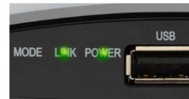
**Step 4D** Wait for a bit as the receiver connects to the **transmitter**. The **LINK** light should be **solid green** once they're connected.
