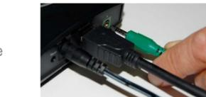
**Step 6C** Remove the protective covering of the double stick tape and attach the flat end of the IR extender cable to the front corner of the HDTV bezel or frame.
